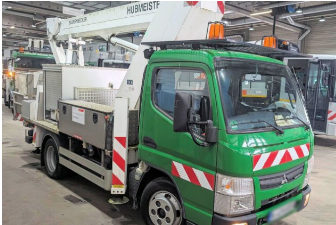
Mitsubishi Canter Fuso 7C15 4x2 Canter Fuso 7C15 4x2, Blumenbecker Hubarbeitsbühne 16m
