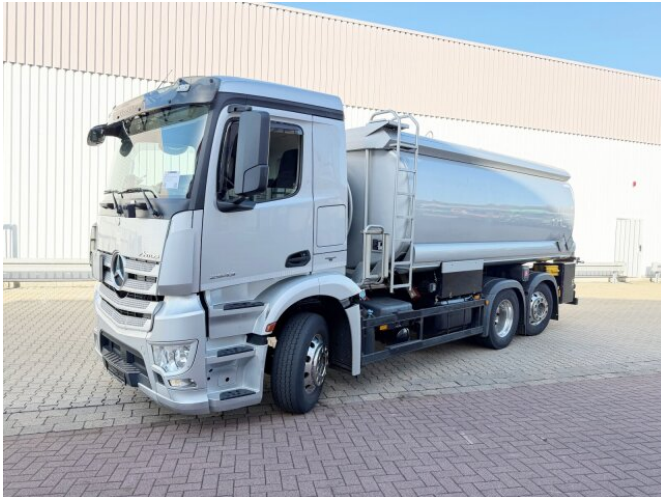
Mercedes-Benz Antos 2543 L 6x2 Antos 2543 L 6x2, Retarder, Lenk-/Lift, Esterer Tank ca. 20m³, 2 Kammern, Funk
