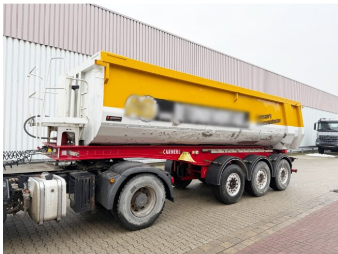
Carnehl CHKS /AH, ca. 26m 3 CHKS /AH, Alumulde ca. 26m 3 , Liftachse
