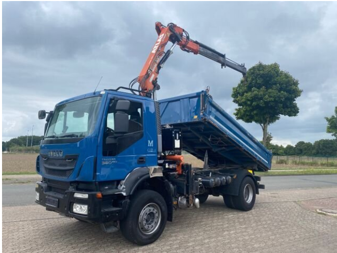
Iveco Trakker AD190T36 4x2 Trakker AD190T36 4x2, EEV, Kran Atlas AK 105.2-A2
