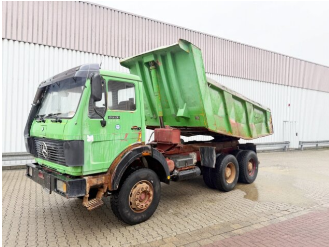
Mercedes-Benz NG 2628 K 6x4 NG 2628 K 6x4, V8-Motor, MEILLER Stahlmulde ca. 10m 3
