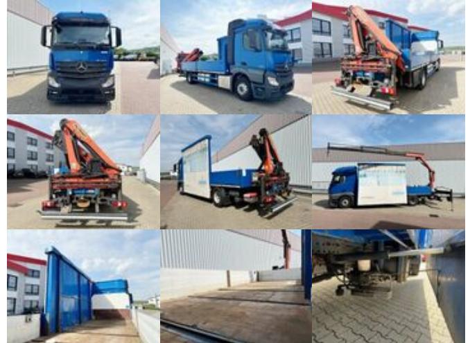
Mercedes-Benz Actros 1836 L 4x2 Actros 1836 L 4x2, Glastransporter, Heckkran Palfinger Pk 12002-EH, Funk
