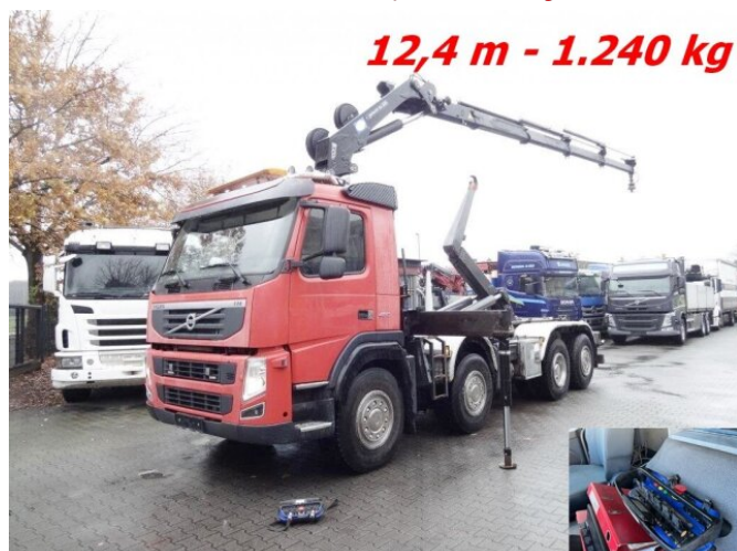
Volvo FM 460 8x2-6 FM 460 8x2-6, Kran HMF 2020-K4, Funk, Lenk-/Liftachse
