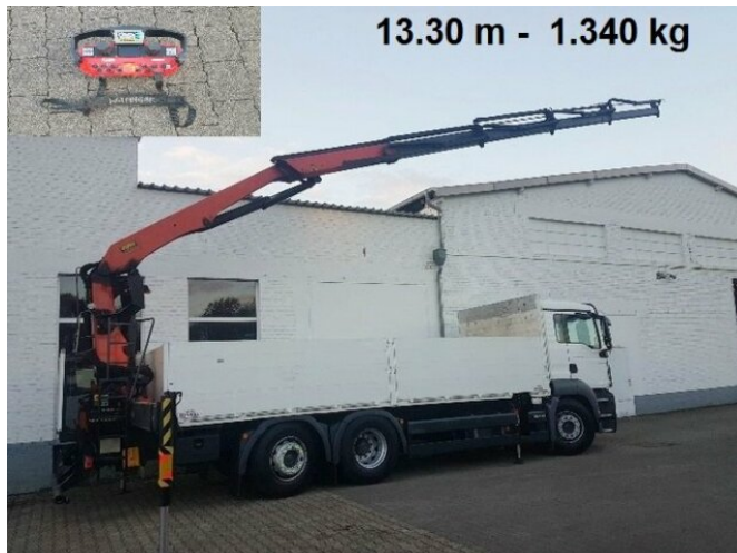
MAN TGS 26.360 LL/6x2/4 TGS26.360LL 6x2,Baustoff,Kran Palfinger PK24001
