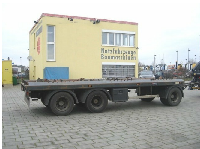
S-K-E-L-M-S-K ASM PA 24 SKELMSK ASM PA24, 2x Anh. f. Absetzcontainer
